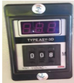
Figura 15. Timer digital 999min asy-3d-110v cnc 9 pines
