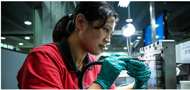
Hand Polishing for the mold
