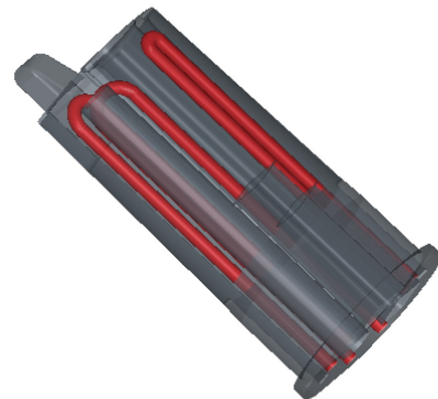
Conformal Cooling Channels made with 3D Printing
