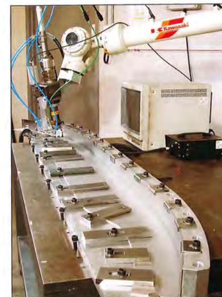
Right The process of Nd:YAG laser beam welding commences.
