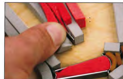
Top This is the steel rule wooden die used for the Libellule light (page 269).
