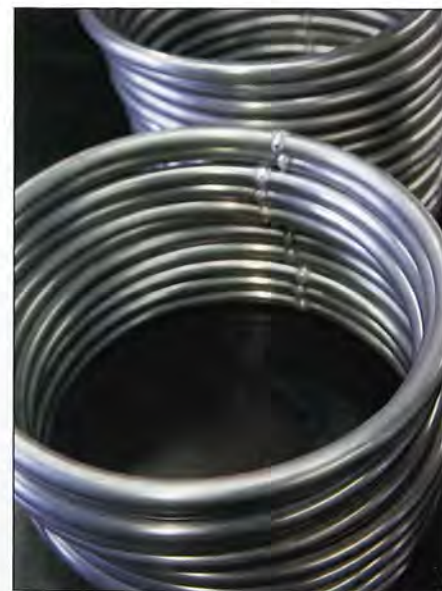
Left Continuous circular metal profiles, such as these heating elements, are produced by ring rolling and then arc welding the seam.
