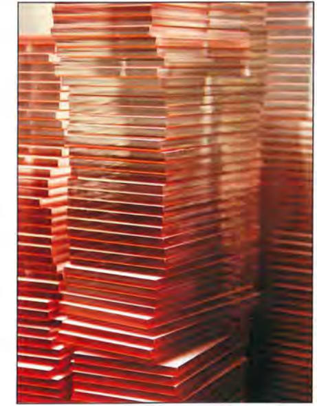
Above Laser cutting produces a polished edge on certain thermoplastics and so eliminates finishing operations.
