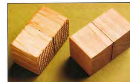
Right These beech blocks have been joined by linear friction welding.
