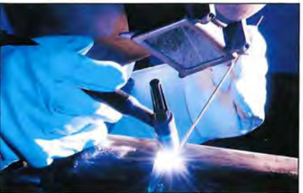
Middle An arc is formed between the tungsten electrode and workpiece, and the filler material melts into the weld pool.
