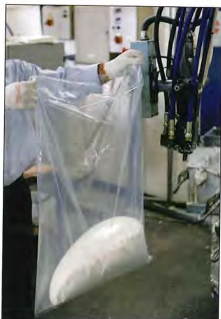
Above The 2 liquids react and expand to form lightweight and flexible foam. The reaction is 1-way, so once the material has been formed it cannot be modified except by CNC machining.
