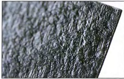
Far left PP and glass fibre have been woven together into a novel composite material, which can then be formed into rigid, lightweight panels using resin transfer molding technology.
