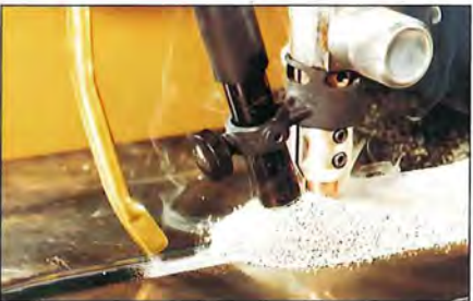
Right In submerged arc welding a solid flux is used, which limits the process to horizontal joints including lap, butt and tee profiles.
