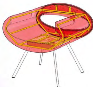
Above The Eye chair is molded in cold cure MDI formulation of around 55 kg/m 3 (3.4 lb/ft 3 ).
