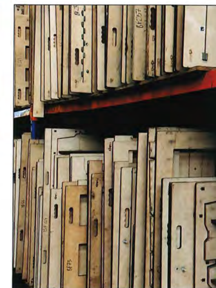
Right These steel rule wooden dies are used to mass produce cardboard boxes and trays.
