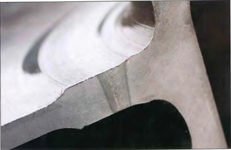
Below This cross-section of electron beam welded joint demonstrates the integrity of a deep weld.
