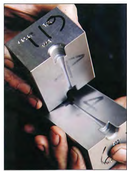
Right Fresh dies are machined from tool steel for each application, because it is uncommon for 2 swaged products to be alike.
