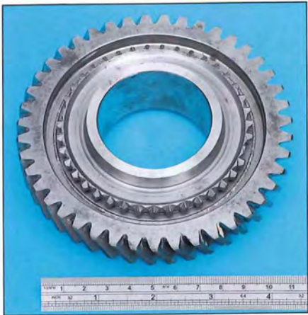
Above The scale of this electron beam welded gear is shown by the ruler beneath it.
