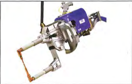
Left Spot welding stainless steel mesh with a handheld welder and larger, static lower electrode. Above Heavy duty handheld welding guns like this are used for general sheet metal assembly work. Sophisticated computer-guided robotic systems are used for high volume welding operations. Below left The welded mesh covers a paper pulp molding tool (page 202).
