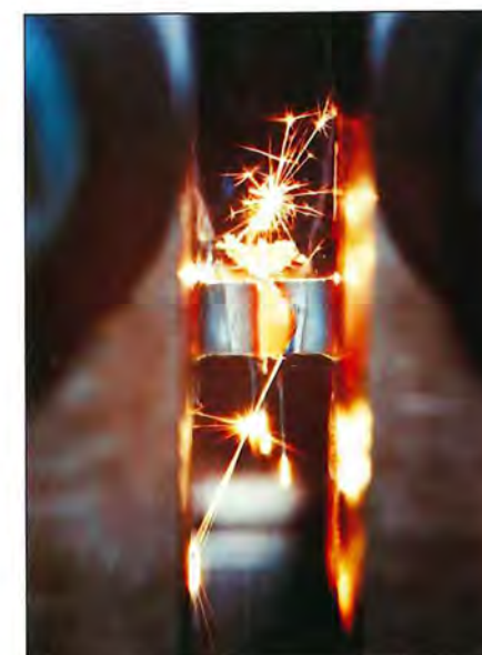
Above This titanium blisk (1-piece bladed disc) for jet engines is made by linear friction welding.
