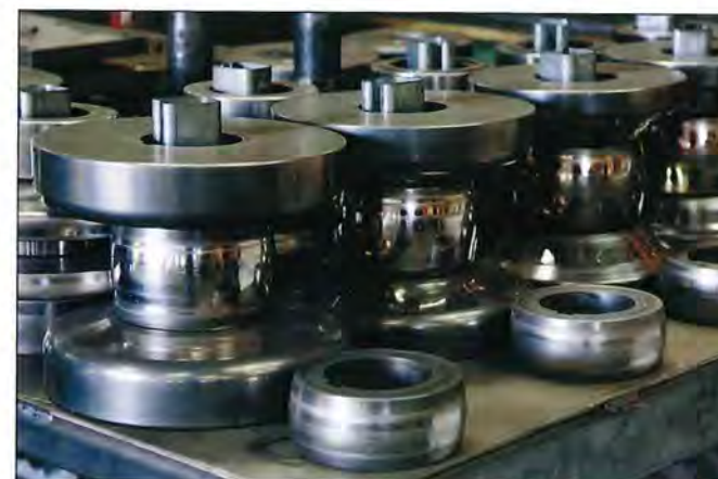
Left Highly polished roll forming tools such as these are used to manufacture continuous metal profiles at speeds up to 4,500 m (15,000 ft) per hour.
