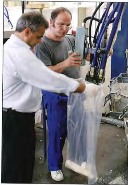
Above A predetermined measure of polyol and isocyanate is dispensed into a plastic bag to demonstrate the reaction process.
