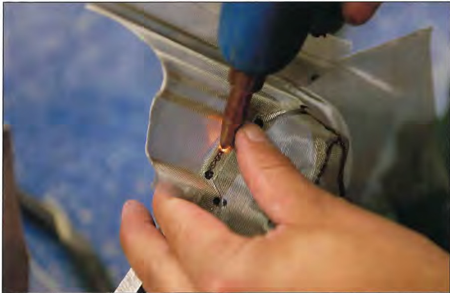
Left Spot welding stainless steel mesh with a handheld welder and larger, static lower electrode. Above Heavy duty handheld welding guns like this are used for general sheet metal assembly work. Sophisticated computer-guided robotic systems are used for high volume welding operations. Below left The welded mesh covers a paper pulp molding tool (page 202).
