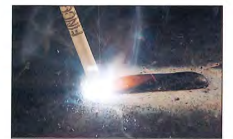
Above left An operator uses MMA welding to join steel plate. Above An arc is formed between the coated electrode and workpiece. Left Joining steel pipes with MMA welding.
