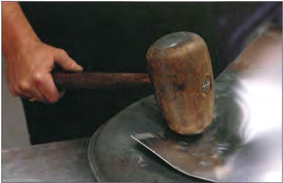
Above Dishing into a sand bag is now largely confined to prototyping.
