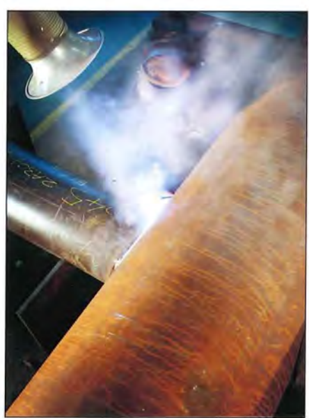
Above left An operator uses MMA welding to join steel plate. Above An arc is formed between the coated electrode and workpiece. Left Joining steel pipes with MMA welding.
