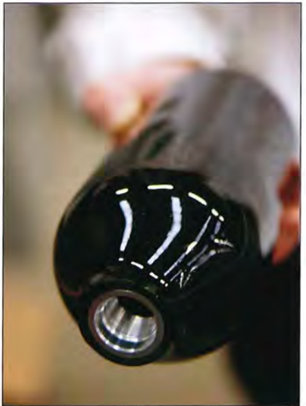
Above This pressure vessel has an aluminium liner filament wound with carbon fibre composite. Left The gloss surface finish is a gel coat resistant to heat or chemical attack. Top CNC machining after filament winding produces very accurate surface dimensions. Channels, recesses and tapers on the outside surface are applied in this way.
