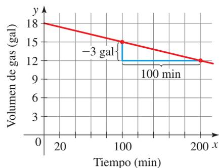
(b) Tanque drenado a 0.03 gal/min
