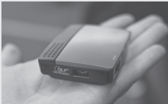
FIGURE 29.9 A prototype pico projector based on DPT. Source: Courtesy of Texas Instruments Corp.
