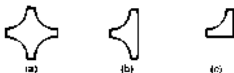
FIG. 9.25 Turret press radius tools
