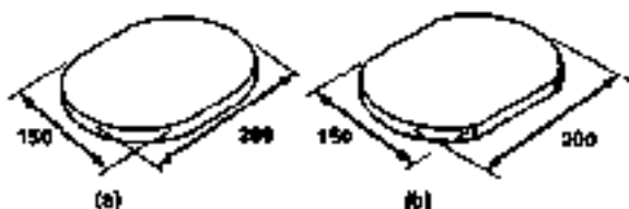
FIG. 9.11 Sheet metal part (dimensions in mm). (a) Blanking design. (b) Part-off design.
